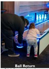
Side ball return allows players to watch the ball being returned and allows operators ease of access to ball return. Safety is key so there is no pinch point at pickup.
